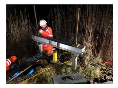
Sacrificial reaction piles were installed to allow the test rig shown in the image above to allow the testing.
